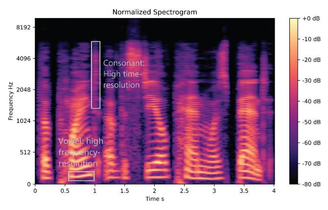
Figure 1: Speech spectrogram illustrating a vowel (lower box) that requires higher frequency resolution and a consonant (upper box) that requires higher time resolution.
